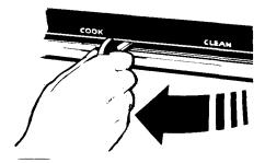
**Step 1:** When LOCKED light is off, slide the LATCH HANDLE to the left as far as it will go and open the door.
